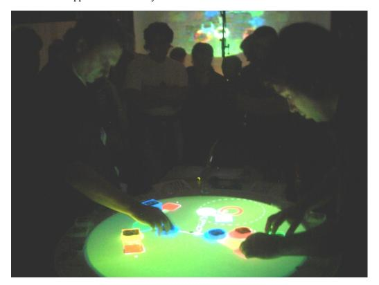
Figure 1: Musicians playing the reacTable\* at Ars Electronica 2005. Objects on the table's surface are tagged with fiducials which are tracked by a camera beneath the table. Some projected graphics represent the telepresence of collaborating performers in Barcelona.
