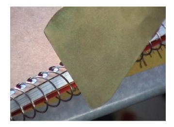
Figure 1: Scraping the wand across the spiral binding of a notebook. The contact between the wand and the notebook causes a continuous acoustic stimulation of the recorded sample.
