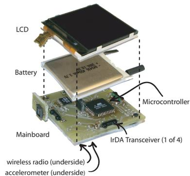
Figure 2. The components of a Siftable computing element
