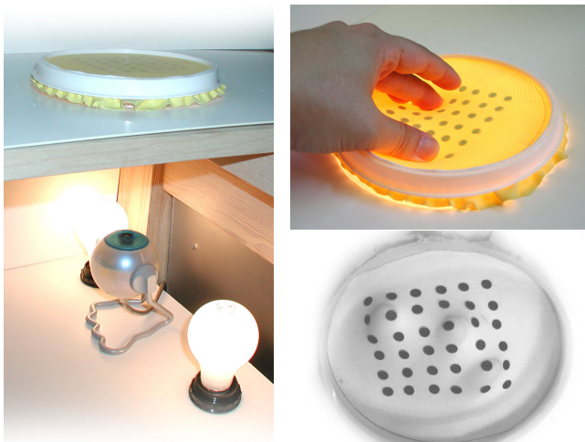
Figure 1: Interface architecture, video camera at bottom (left); interaction with surface (upper right); view as seen from camera (bottom right)
